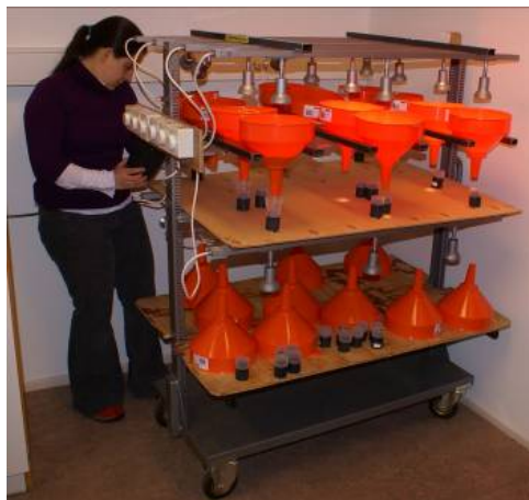
Fig. 7. The Tullgren Funnels at UNIS. being operated by UNIS and University of Bergen Ph.D. student María Luisa Ávila Jiménez. (S.J. Coulson)
